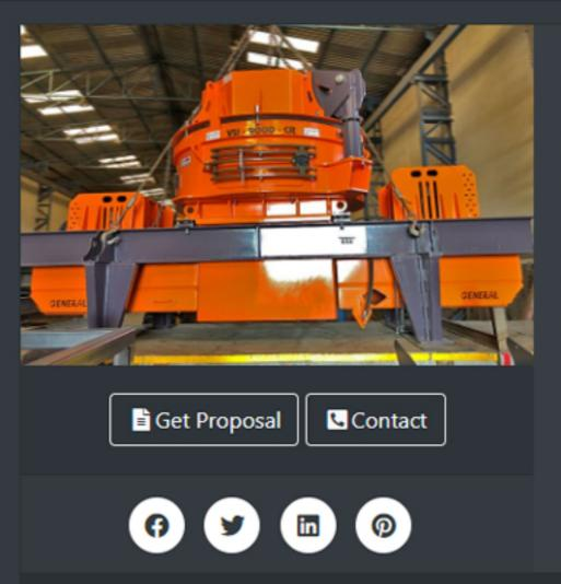
General Machinery Vertical Shaft Impact Crusher (VSI) are used in mining and building sector, breaking all kinds of medium-size hard abrasive materials to get sand and gravel. It is used to get 0.5 mm sand and gravel. Their sand and cubic ratios are high. Spare parts costs are very low and which is a low cost crusher type.
